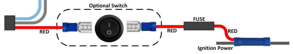
If the installer wishes to be able to switch the controller on and off, install the supplied switch on this wire by cutting the wire and installing the two supplied spade terminals. Installing this switch is optional but is recommended.
