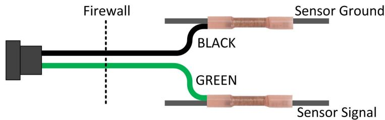
Soldering this particular connection is highly recommended. Alternatively, the installer may wish to utilize two of the provided butt connectors containing integral heat shrink tube. Ensure these two connections are water tight when complete so as to not compromise the original wiring or the sensor output.
